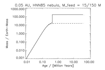
Figure 4: Total mass (full line) and core mass (dashed line) of a Pegasi-planet forming at 0.05 AU from a solar mass star. The accumulation of a gaseous envelope surrounding a condensible element core that grows by planetesimal accretion is shown for the first 100 Mio years. The structure of the envelope is calculated dynamically including time-dependent theory of convection that is calibrated to the Sun and including detailed equations of state and opacities.
